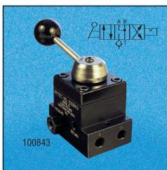
This 4-way, 3-position valve has a center position that blocks the pressure (P) port and drains the two work (A and B) ports back to the tank (T) port. This configuration makes it ideal for an inexpensive double-acting manual pallet valve when used in conjunction with a Hytec pilot operated check valve and any constant pressure pump.
