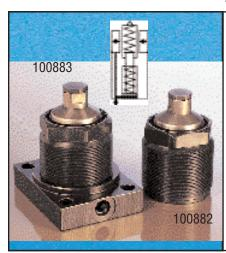
Hyteo's fluid advance work supports have a spring loaded plunger which hydraulically extends to contact the workpiece. To support any externally applied loads, the sleeve surrounding the plunger grips the plunger and holds it in place.
