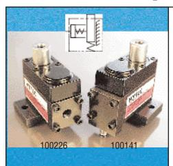
Work supports provide the stability that prevents deflection and vibration of the workpiece during machining. Automatically adjustable to varying sizes or positions of the workpieces, they are also usable as adjustable rest pads under clamps.
