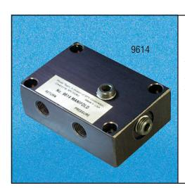
The 9614 manifold assembly comes as standard equipment on Hytec pumps No. 100186, 100280, 100190, 100200, 100174, 100220 and 100211. It provides the connection points for pressure and return lines as well as a gauge and/or pressure switch. These pumps are designed to have this manifold removed and directly replaced by our number 9504 pump-mounted control valve.
