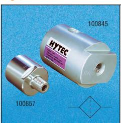
No. 100845 - This high pressure filter is intended for use in systems where there is flow in only one direction such as pressure or return lines between the power source and control valve. This in-line filter has a removable/replaceable sintered bronze element. The element is accessible without removing the filter body from the installation.
