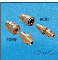
Hytec offers both an economical standard poppet type coupler and labor-saving push-to-connect flat face coupler. Both styles are rated at 5,000 psi that has ¼" NPTF connections.
