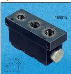
Hyteo's pilot operated check valve offers a unique poppet seal design making them ideal for pallet applications or other specialized control circuits where zero leakage is essential. They can be used in any application where pressure must be maintained in a portion of a circuit until a separate pilot signal opens the valve and allows free flow in the reverse direction.
