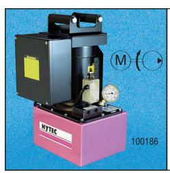
These electric/hydraulic pumps are twostage, continuous pressure (demand) pumps that contain all the necessary controls and circuitry for powering any single- or doubleacting continuous pressure workholding system. They have a pressure switch and an external pressure regulator, both infinitely adjustable throughout the operating pressure range of 1,000 to 5,000 psi. An internal safety relief valve prevents damage from exceeding the maximum rated pressure.
