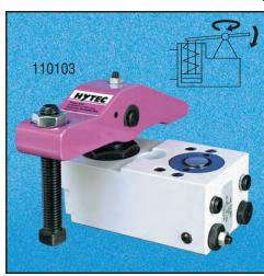
Single-screw mounting and the adjustable clamping screw make these clamps easy to reposition on the fixture to adapt to various workpiece sizes, and make set-up and adjustment faster than other methods. It also lets you clamp several workpiece sizes without changing the fixture each time. When mounted on a T-slot machine table, the need for fixtures is often eliminated.
