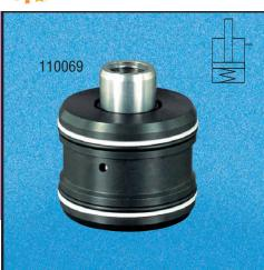
These cylinders retract when hydraulically pressurized to exert a pulling force on clamping elements or mechanisms. For straight pull applications only, they allow the user to design a cylinder into a fixture while maintaining the replaceability and long life of a heat treated, corrosion resistant cylinder body. Designed for single-acting systems only, the cylinder's return spring is built into the piston and requires no additional fixture space.
