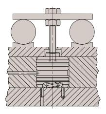
Required thickness will vary due to fixture material used. Must resist maximum cylinder force.
