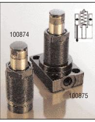
Hytec's spring advance work supports have a spring loaded plunger which contacts the workpiece as it is loaded into the fixture. The spring keeps the plunger in contact with the workpiece, allowing for variations between workpieces. To support any externally supplied loads, the sleeve surrounding the poppet grips the plunger and holds it in place.
