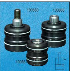
These "Pull" cylinders retract when hydraulically pressurized. They were created to permit the user to design a cylinder into a fixture while maintaining the replaceability and long life of a heat treated, corrosion resistant cylinder body. Typical applications of these cylinders include installation behind fixture plates or buried in tombstones where they can supply clamping force without taking up valuable fixture space.
