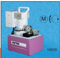
This electric/hydraulic pump is a two-stage, continuous pressure (demand) pump that contains all the necessary controls and circuitry for powering any single- or double-acting continuous pressure workholding system. It has a pressure switch and an external pressure regulator, both infinitely adjustable throughout the operating pressure range of 1,000 to 5,000 psi. An internal safety relief valve prevents damage from exceeding the maximum rated pressure.
