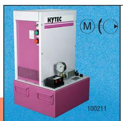
These electric/hydraulic pumps are twostage, continuous pressure (demand) pumps that contain all the necessary controls and circuitry for powering any single- or doubleacting continuous pressure workholding system. They contain a pressure switch and pressure regulator that are infinitely adjustable throughout the operating pressure range of 1,000 to 5,000 psi.
